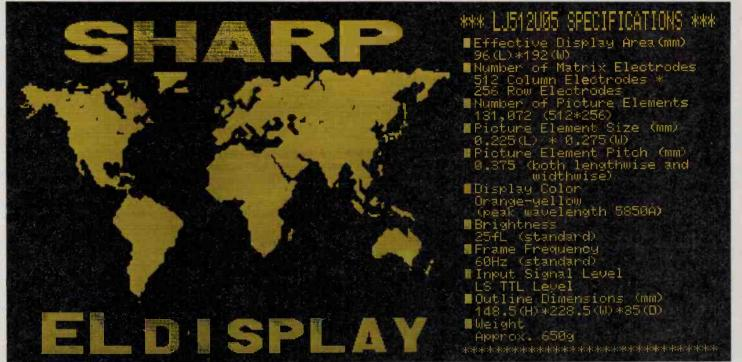
Sharp's full line of EL (Electro Luminescent) Displays are thin (34mm), lightweight (650 grams), low power (15 watts max) and the two latest editions can display 25 lines of 80 characters. These "State of The Art" Displays feature; line by line scrolling, blinking characters, full graphics and a
