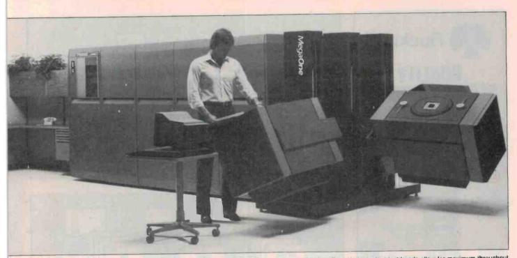
The MegaOne system. Using a complete tester for each pin, it can test VLSI devices with up to 256 pins. Three independent test heads allow for maximum throughput.
